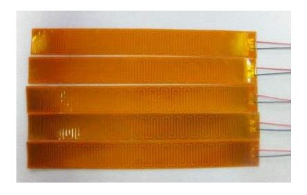
A. The heating function adopts BMS to control the heating film, and the protection plate can start the heating mode by collecting the temperature and current;
